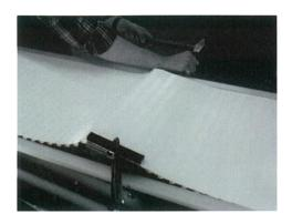
2. Rod removal can be easier by supporting opposite belt edge with fixing tool, such as shown in picture below.
