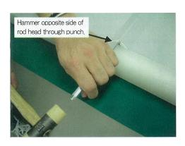
4. If you do not have a fixing tool (such as shown in picture of step 2), hold opposite belt edge as shown in picture below.
